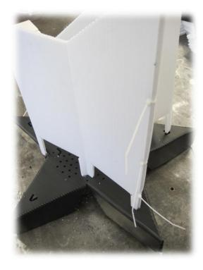
flat bottom edge of the star is flush with the base of the star. It is normal for the legs to be tight in the slots, so it may be necessary to pull on the legs from the bottom of the star to get them to completely "seat" into the slots.
