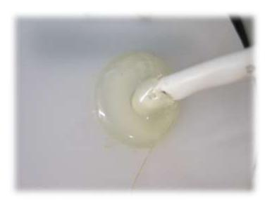
12. Put a moderate amount of hot glue around the top of the cap where the CAT5 cable enters the cap. Hold it there for about 30 seconds or until the hot-glue has setup. It should look like the photo to the left.
