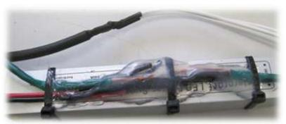
other indicator (we use fluorescent pink tape) to the long end of the CAT5 cable that has power output (the end that was wired to the power supply.) The power output side will provide power to the entire chain of MegaBalls until it "hits" another power injector for another 10 balls.
