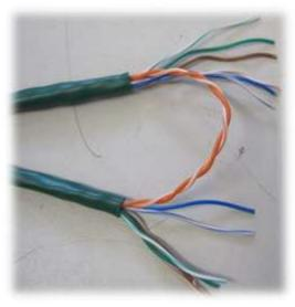
color wires (green, blue, brown) together and then twist all the striped wires together (green/white, blue/white, brown/white) so that all the ends of the wires are touching each other as shown to the left:
