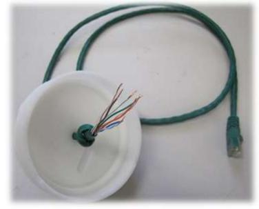
6. Just like the power supply, twist all the solid color wires (green, blue, brown) together and then twist all the striped wires together (green/white, blue/white, brown/white) so that all the ends of the wires are touching each other and then solder them together. Also apply a small amount of solder to the orange and orange/white wires. Trim and excess length so that only about 1/8" of exposed wire that has been soldered remains.
